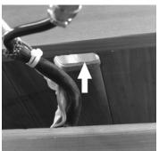
6. With the lid in place remove the (4) screws to access the power supply unit.
